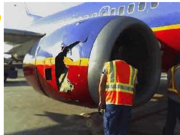
Southwest Airlines Fan Disk Failure
