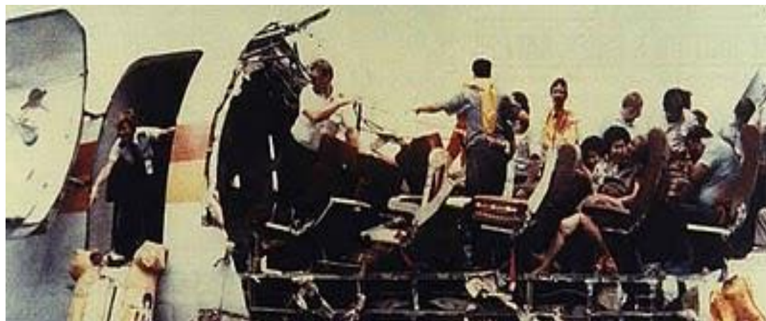
4-28-1988 After 89,090 flight cycles on a 737-200, metal fatigue
