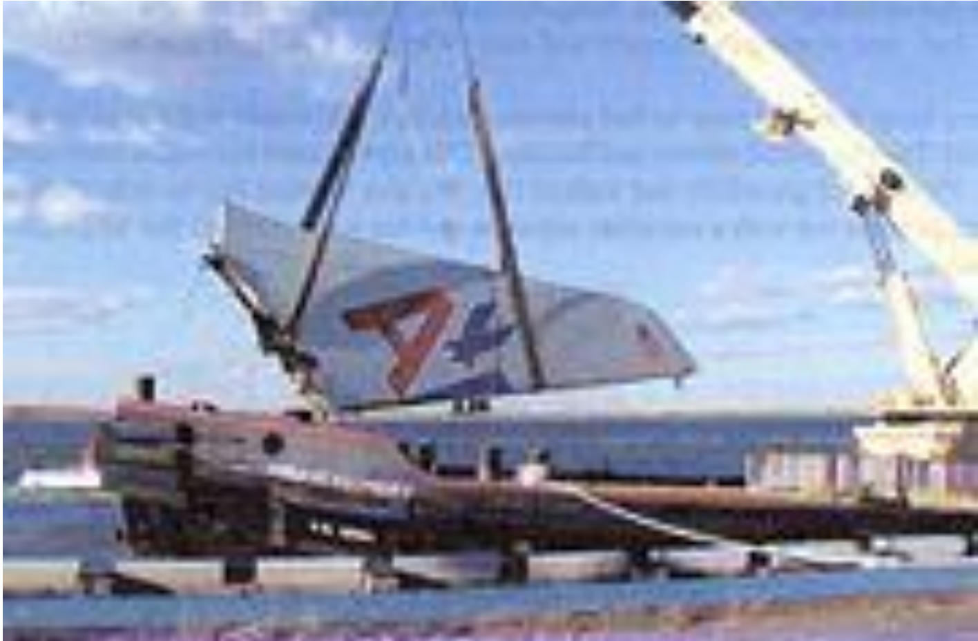
American Airlines Flight 587 Vertical Stabilizer
