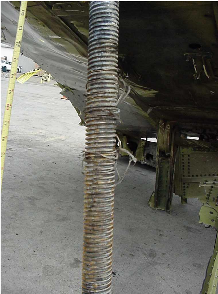
Alaska Airlines Flight 261 Horizontal Stabilizer Jackscrew
