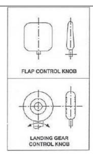
(d) If conventional powerplant control knobs are used by the UAV crew, they must conform to the general shapes (but not necessarily the exact sizes of specific proportions) in the following figures:
