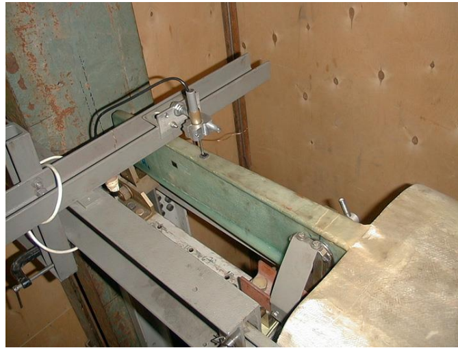
Fatigue stand of the glider wing spar
