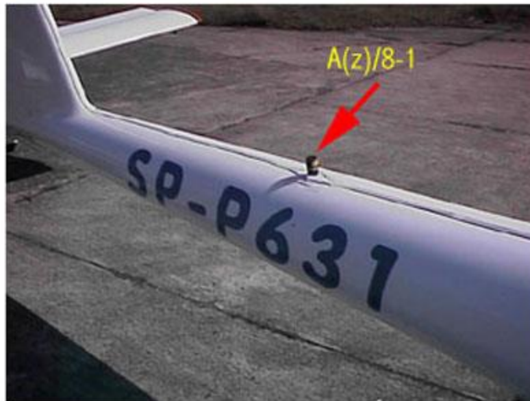
Photos of accellerometers and deflection transducer fixed on the gl
