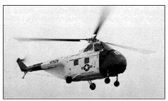
advances in helicopter design. These aircraft had a large cabin under the rotor, and to give a wide allowable center of gravity position, the engine was placed in the nose. Westland also maintained their relationship with Sikorsky and built versions called the S-55 Whirlwind and S-58 Wessex.
