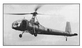
During 1944, the Cierva-Weir Company, prompted by the initial success of Sikorsky's R-4 and R-5, proposed a rather large single-rotor machine called the W-9. This machine was rather unique in its use of jet thrust to counteract rotor torque reaction -- see Everett-Heath (1986). However, because the rotor lacked any collective pitch control, rotor thrust was
