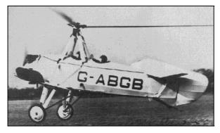
Although de la Cierva's autogiro was still not a direct-lift machine and could not hover, it required only minimal forward airspeed to maintain flight. Juan de la Cierva proved that his autogiros were very safe and essentially stall-proof, and because of their low speed handling capability, they could be landed in confined areas. Takeoffs required a short runway, but this problem was solved with
