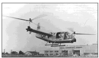
The tilt-rotor aircraft takes off and lands vertically with the rotors pointed vertically upward like a helicopter. For forward flight, the wing tip-mounted rotors are progressively tilted to convert the aircraft into something that looks like a fixed-wing turboprop airplane. In this mode, the tilt-rotor is able to achieve considerably higher flight speeds (about 300-kts; 555-km/h;
