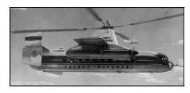
In Great Britain during the 1940s and 50s, the autogiro concept was pursued to some significant end by the Fairey Aviation Company. The Fairey Girodyne compound aircraft used a propeller set on the end of a stub wing to provide both propulsion and antitorque; see Everett-Heath (1986). The Fairey Company went on to
