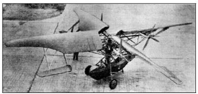
lift on the blade as it swept around the rotor disk. For vertical flight, the tabs on all the blades moved collectively to increase the rotor thrust. Three small propellers mounted to the airframe were used additional pitch, roll, and yaw control. This machine held modest FAI speed and altitude records for the time, including altitude (57 ft, 17.4 m), duration (8 minutes 45 seconds) and distance flown (3,589 ft, 1,078 m).
