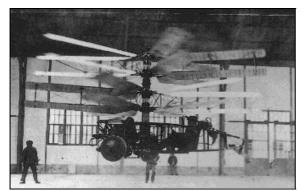
During the early 1920s, Raul Pescara, an Argentinan living and working in Spain and France, was building and attempting to fly a coaxial helicopter with biplane-type rotors. On his first machines, each rotor had four sets of biplane blades that were mounted rigidly to the rotor shaft, and this was later increased to a remarkable five sets per rotor, giving a total of 20 lifting surfaces. As described by Boulet (1984), Pescara's work
