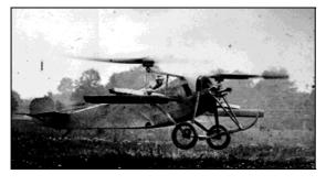
In the United States, Emile and Henry Berliner (a father and son) were interested in vertical flight aircraft. As early as 1909, they had designed and built a helicopter based on pioneering forward flight experiments with a wheeled test rig. They were one of the first to observe the fact that the rotor power required for hovering flight was substantially greater than for flight at low forward speeds.
