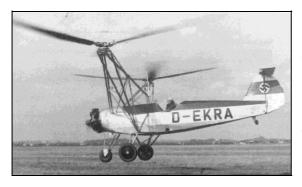
Heinrich Focke of the Focke-Wulf Company began his work on rotating-wing aircraft as early as 1933. He acquired a license to build de la Cierva's autogyros, and successfully manufactured the C-19 and the C-30 models. From the experience he gained by working on these machines and after many wind tunnel tests with small models, Focke began developing the FW-61 helicopter in 1934, named after his current
