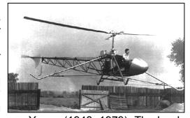
invented a teetering rotor with a stabilizer bar; see Young (1948, 1979). The bar had bob weights attached to each end and was directly linked to the rotor blades through the pitch control linkages. The idea was that if the rotor was disturbed in pitch or roll, the gyroscopic inertia of the bar could be used to introduce cyclic pitch into the main rotor system, increasing the effective damping to disturbances and giving stability to
