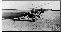
In the late 1920s, the Austrian engineer Raoul Hafner designed and built a single-seat helicopter called the R-2 Revoplane -- see Everett-Heath (1986) and Fey (1987). The flights were mostly unsuccessful despite some brief tethered flights of up to a minute. His early machines used a
