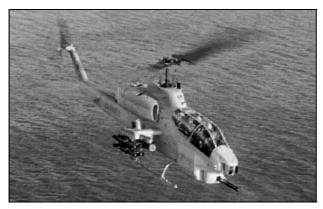
The success with the Model-47 led Bell Helicopter to develop the UH-1 Huey, which were delivered starting in 1959. The Bell 212 was a two-engine development of the UH-1D, and proved to be a successful military and civilian machine. The Huey-Cobra also grew out of the UH-1 series, retaining the same rotor components, but having a more streamlined fuselage with the crew seated in tandem. The type is still in
