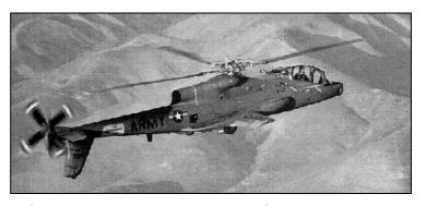
addition, the high parasitic drag of the rotor hub and other airframe components leads to a relatively poor overall lift-to-drag ratio of the helicopter. This generally limits performance of conventional helicopters to level-flight cruise speeds in the range of 150 kts (278 km/h; 172 mi/h), with dash speeds up to 200 kts (370 km/h; 230 mi/h). Although somewhat higher flight speeds are possible with compound designs, which
