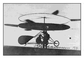
About 1914, the Danish aviation pioneer Jen C. Ellehammer designed a coaxial rotor helicopter. Boulet (1984) gives a good description of the machine. The rotor blades themselves were very short; six of these were attached to the periphery of each of two large circular aluminum rings of about 20-ft in diameter, with the wings extending out about another 5-feet. The lower disk was covered with fabric and was intended to serve as a parachute in the event the blades or the
